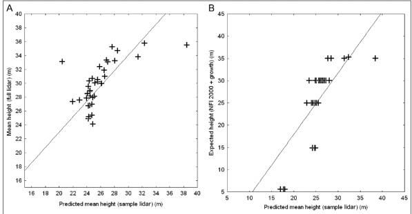
**Figure 5.** Height prediction using the image segmentation-based model: (a) predicted mean height (sample lidar) versus mean height observed from full lidar coverage, and (b) predicted mean height from sample-based lidar versus inventory heights (last NFI + growth obtained from SI-curves).
