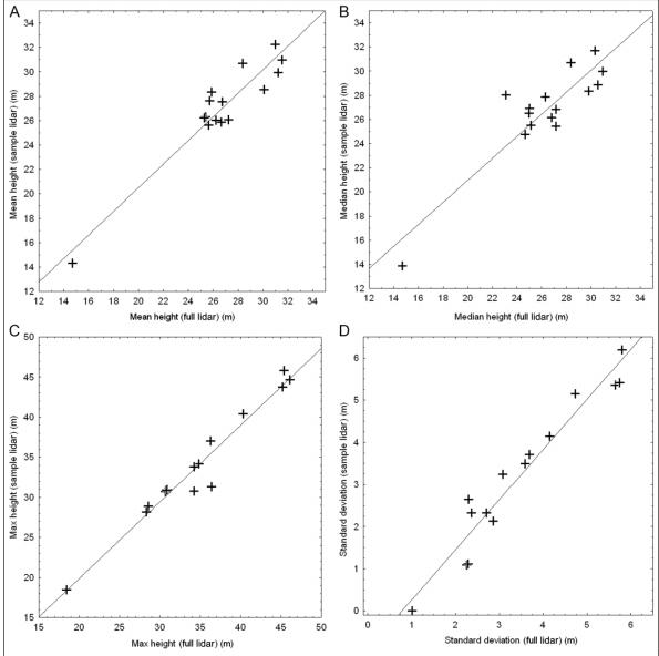
**Figure 4.** Correlation between transect lidar and full-coverage lidar data for (a) average maximum height, (b) median height, (c) maximum height, and (d) standard deviation.
