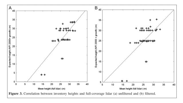
(R = 0.78, p < 0.05) and, importantly, a *t*-test confirmed that the stand height estimates are not statistically different (p > 95%).
