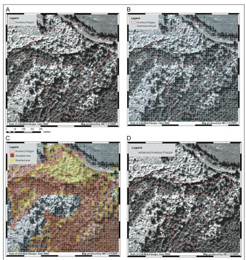
**Figure 2.** Adjusting spatial scale of inventory boundaries within forested areas using the lidar filter: (a) original inventory polygon, (b) superimposed grid, (c) rejected and accepted areas, and (d) redefined inventory boundary.
