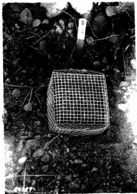
Plate 6. Depth guide removed and cage placed.
