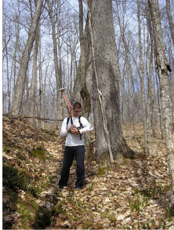
Figure 3. Recording the centre of a tree crown in Swan Lake with the Trimble ProXT and Hurricane antenna on a 'ruggedized' laptop.
