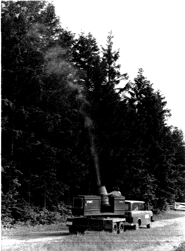
Figure 1. Application of permethrin by FMC Rotomist® 100HT for the control of spruce budworm on white spruce near Grand'Mère, Que.
