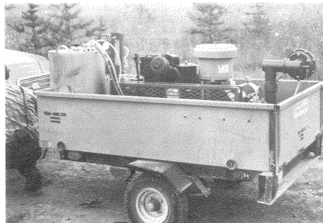
Figure 1. Leco ULV cold fog generator Model HD.
