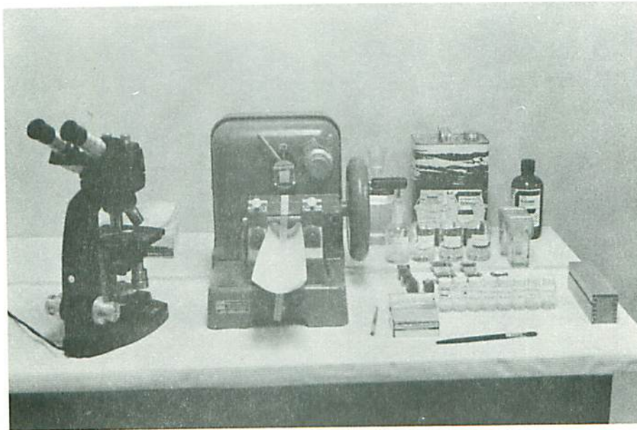
Fig. 1(b) Paraffin sectioning with a Rotary Microtome. The paraffin ribbon containing the sections were lifted up on a paper and then gently placed on the slides.
