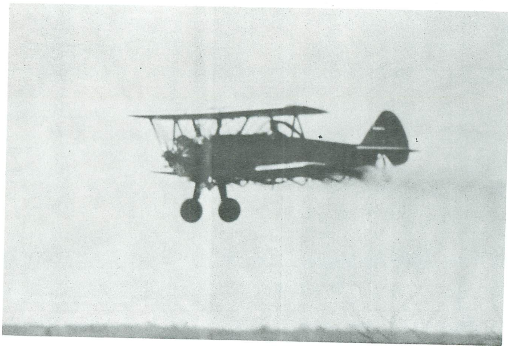
Figure 5. Application of methoxychlor at 4 gallons spray mixture per acre.
