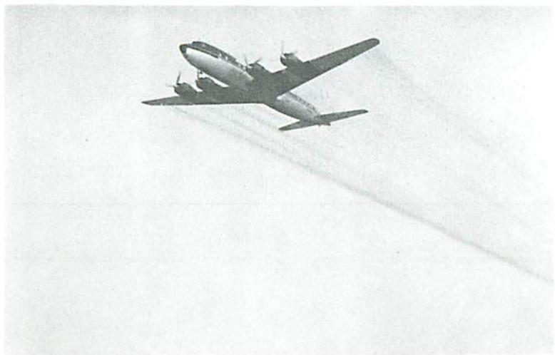
(c) Front view of the DC-7 showing spray emission and spray cloud formation.
