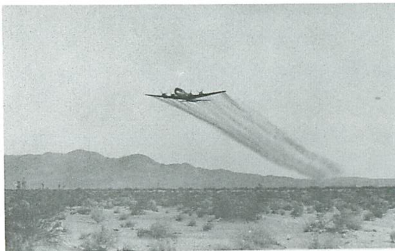
(b) Cone shaped spray cloud resulting from mixing of the wing- tip vortice and propeller slipstream
