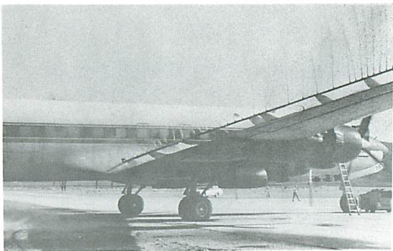
Fig. 4 (a) Side view of the DC-7 during stationary spray emission at airport.
