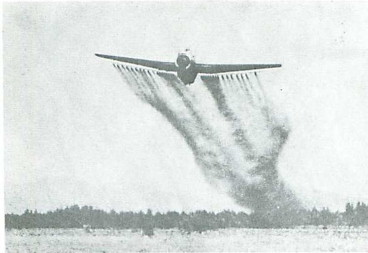
Fig. 9(a). Picture of spray cloud characteristics produced by vortice effect from single engine aircraft.
