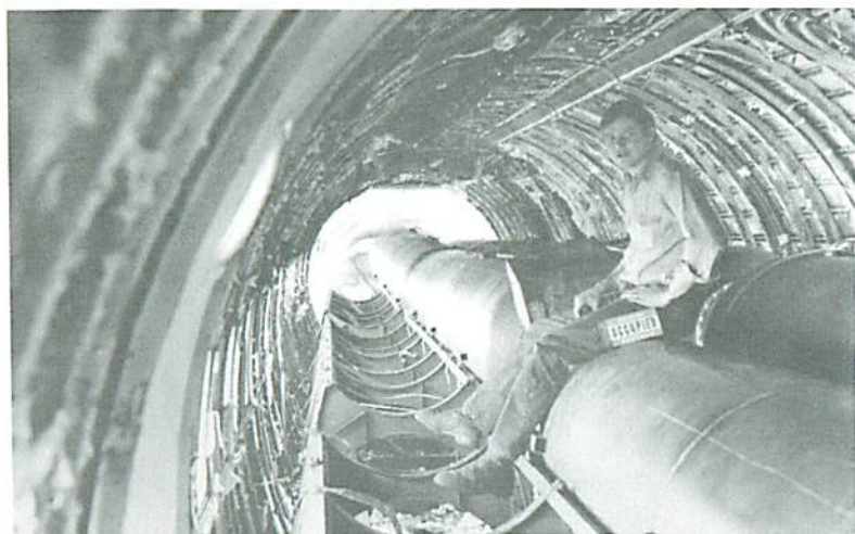
Fig. 2 (a) Interior view of DC-7 showing tank mount bracket (left) and mounted tank (right)
