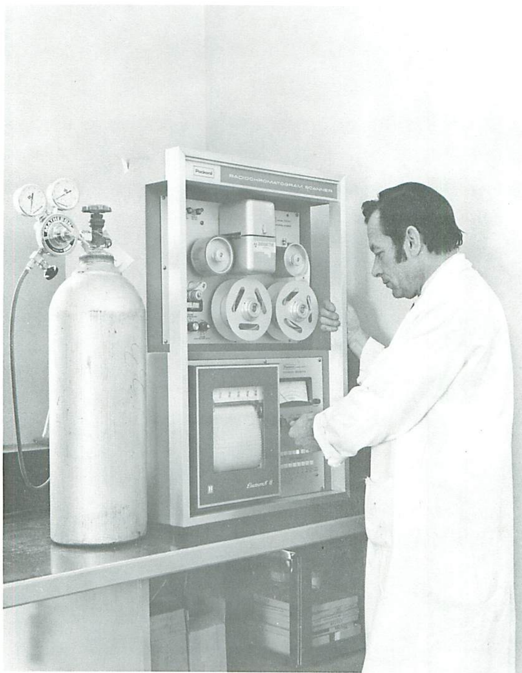
Fig 6 Chromatogram scanner for the estimation of isotopically labelled pesticides and their metabolites.
