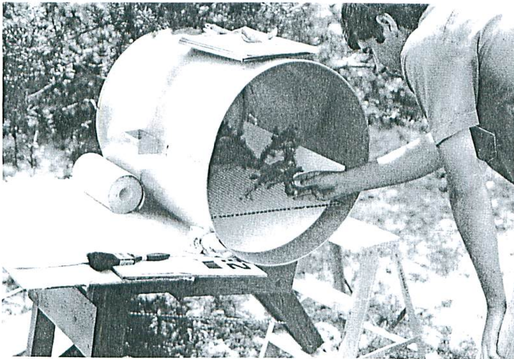
Fig. B-2 Modified use of the sampling apparatus for determining larval densities on branch samples
