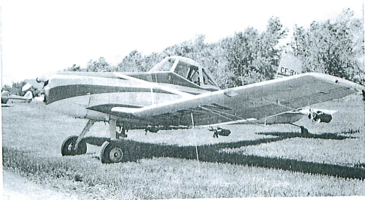
Fig. C-4 The Cessna Agwagon spray aircraft fitted with Micronair AU 2000 units
