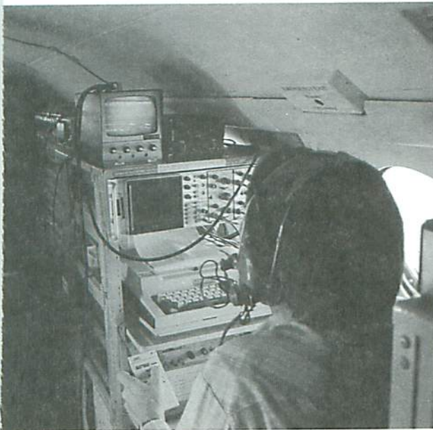
Information gathered by a Multi-Spectral Imagery Scammer is helping foresters determine the health, tree species and harvest potential of the forest.
