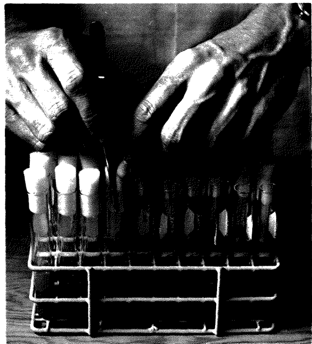
FIGURE 1. Forceps-plugging of racked agar slants with polyfoam plugs.
