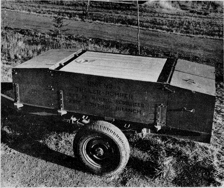
FIGURE 3—Tanker-trailer from which tank can be readily lifted out.
