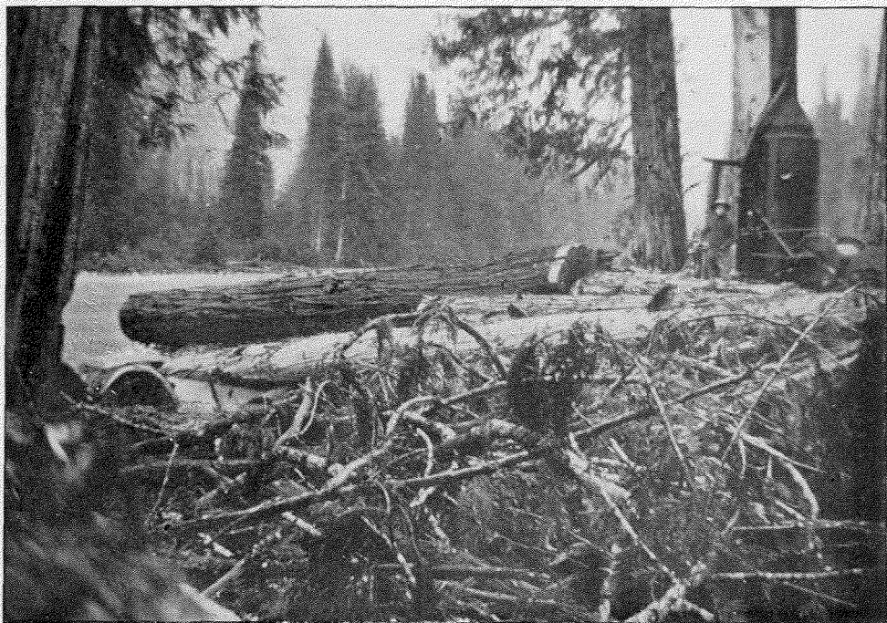
On Fish River, B.C., showing Cedar Logs and Donkey Engine used in drawing logs and water.
