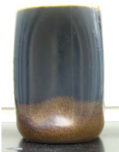
Figure 1. Diluted weak black liquor (14.5% solids) received from Mill E clearly shows a light brown “sinking soap” phase at the bottom of the container.
