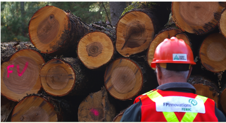
Inspecting hardwood log pile for potential veneer logs
