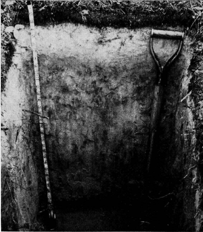
FIGURE 10. A Sandy Gley Podzol with the summer level of the ground water table at 3.5 feet. Note the strongly developed A_0 and A_2 horizons and the mottled, gleyed B and C layers.
