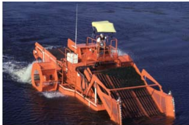
Figure 2. Specially designed mowing equipment for cutting submersed aquatic plants.
