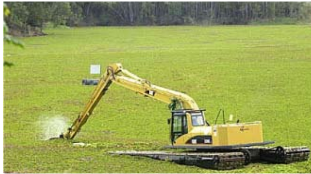
Figure 1. Floating backhoe removing salvinia from an infested lake.
