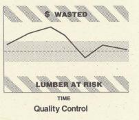
tor treatment levels and even determine how uniformly individual boards have been treated. This means that an in-mill quality control program will soon be possible. Surface treatment of green lumber by DDAC is required for sap stain control. Surprisingly, rough wood, which has many times more 'wood fiber surface'/cm<sup>2</sup> than smooth wood, does not require any more DDAC measured as µg per cm<sup>2</sup>.
