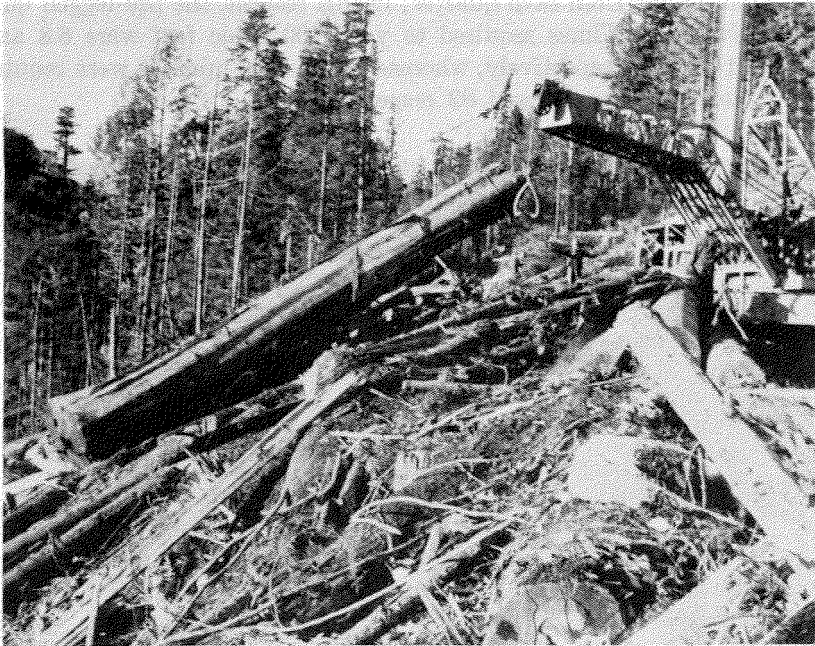
FIGURE 9—A pre-log largewood cedar butt log is yarded to the landing.
