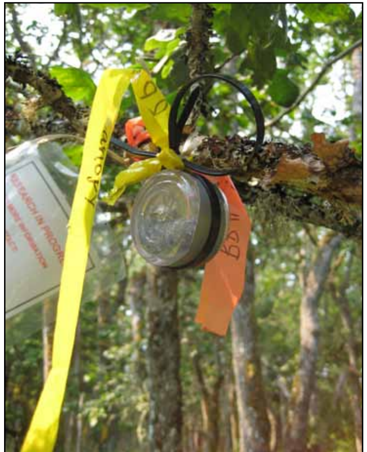
P124-09. iButton DS1922 datalogger on branch.
