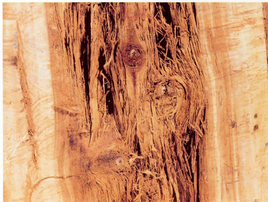
Fig. 42 Red-brown stringy trunk rot caused by the Indian paint fungus, Echinodontium tinctorium .
