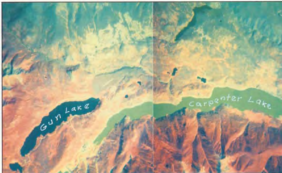
Figure 16. Color composite imagery produced from band-filter combinations on color additive viewer from high-altitude (9450 m ASL) airborne MSS - a combination of bands 4, 10 and 11, projected through blue, red, and green filters, respectively.
