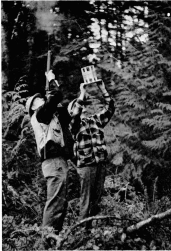
Development of a special line-gun to obtain samples from crowns of tall trees.
