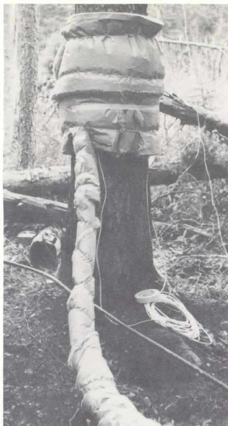
Insulated coils containing chilled antifreeze controls flow of sap during tests to determine ability of the tree to resist invasion of blue stain fungi introduced by bark beetles.
