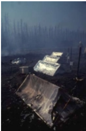
Figure 3—Fire shelters were placed at varying distances from the edge of the crown fire plots. The fire shelter in the foreground was 2 meters from the plot's edge.
