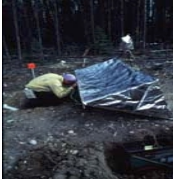
Figure 2—Setting up a fire shelter for testing during the International Crown Fire Modeling Experiments in the Northwest Territories during 1998
