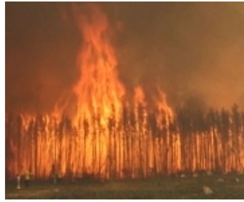
Figure 6--Plot 4 fire. Note that the fire has nearly reached the edge of the fuel and is not forming a uniform flame front.
