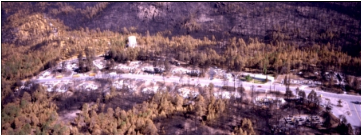
Photo 6—Significant structure-to-structure fire spread occurred from flames and firebrands in an area of multifamily residences. The unconsumed vegetation surrounding the corridor of destruction indicates that the high fire intensities were due to the burning structures.
