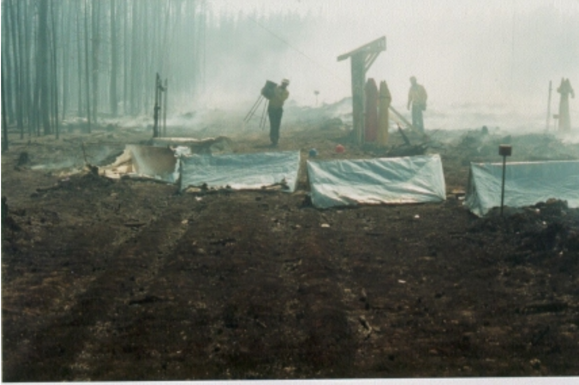
Figure 7 Post Burn Photograph of Fire Shelters Deployed on the Down Wind Edge of Plot 8
