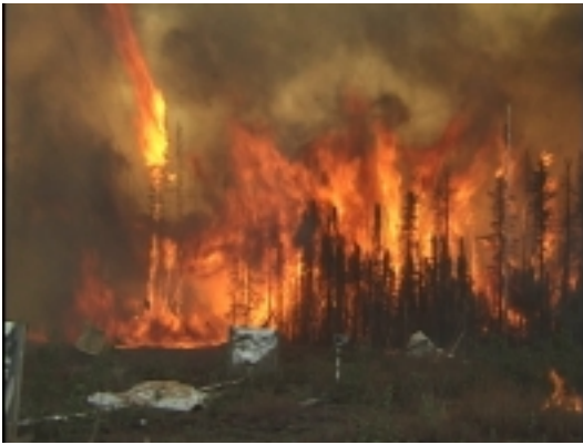
Figure 4--Plot 1 fire. This fire was characterized by torching rather than a coherent uniformly spreading flame as a function of separation distance.
