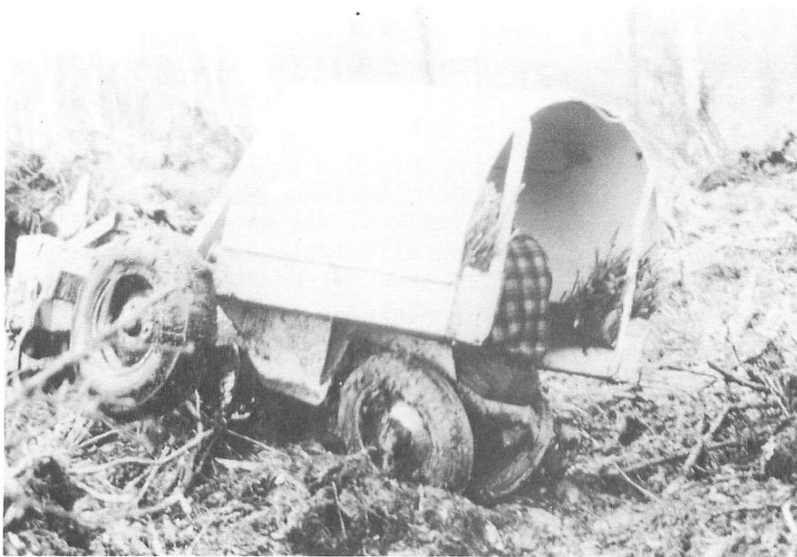
Figure 3. The Reynolds-Lowther Crank Axle Planter
