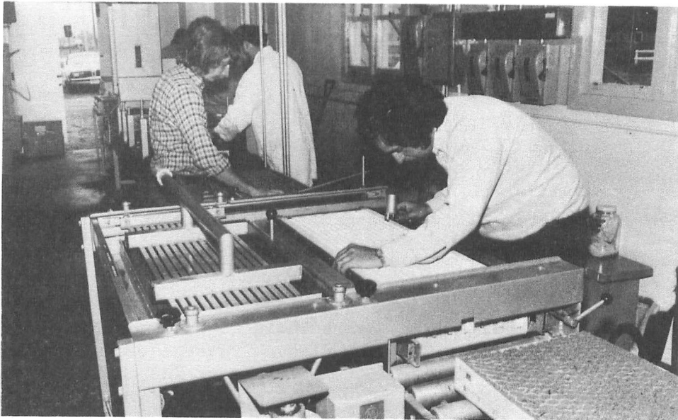
Figure 5. Seeding of containers on semi-automatic Japanese paperpot production line.
