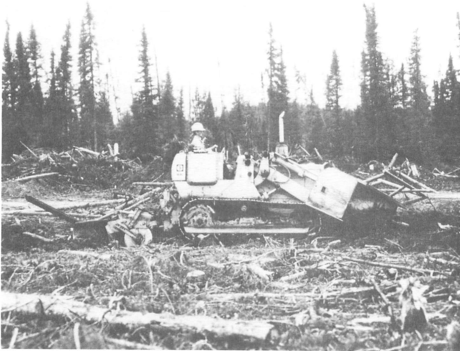
Figure 2. The CFS seeding assemblage without the trailing seeder.
