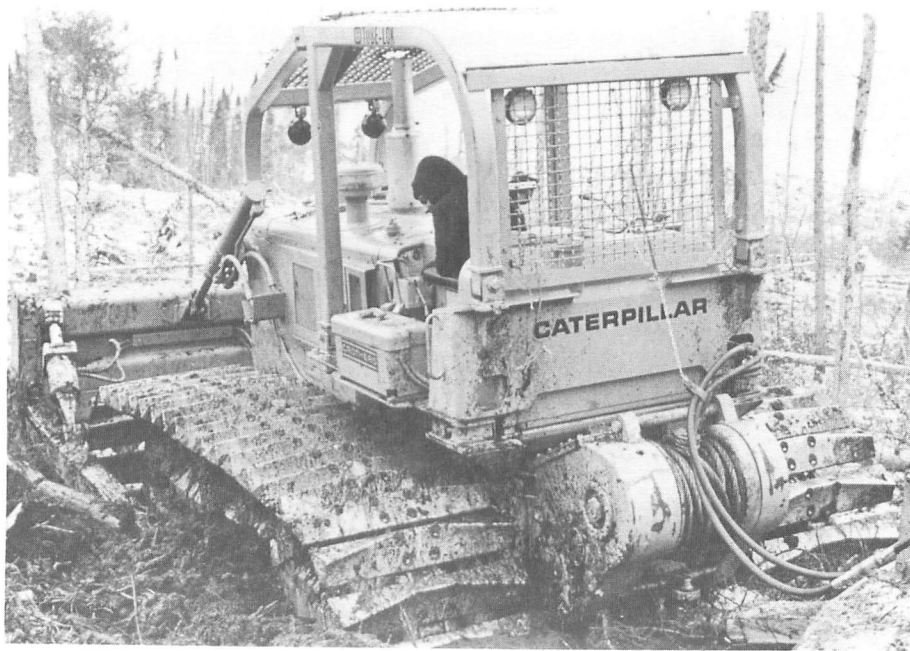
Figure 1. High-flotation crawler tractor of the kind necessary for traversing wet or soft-soiled areas during site-preparation operations.
