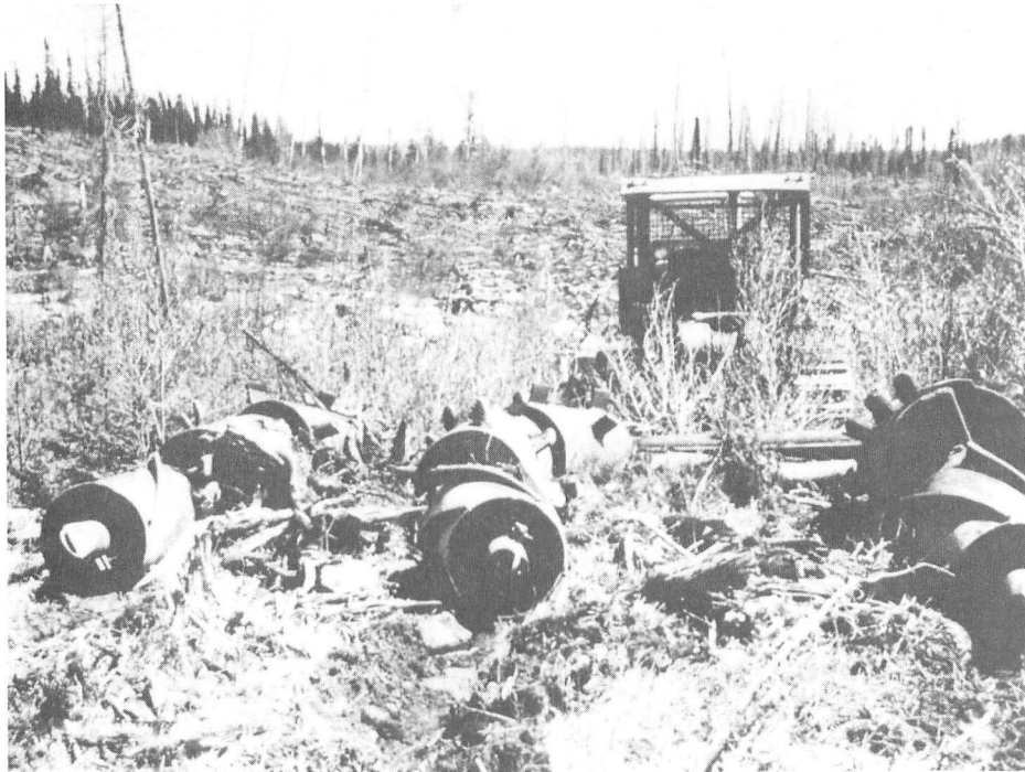
Figure 1. The barrel seeder with three scarifying barrels and three trailing seed barrels.
