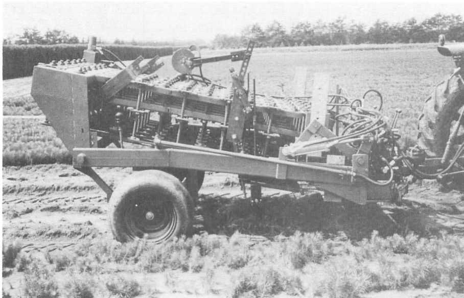
Figure 1. First prototype of semi-automatic seedling harvester being developed jointly by OMNR and GLFRC.
