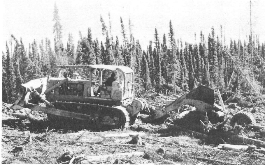
Figure 1. The Marttiini KLM-240 Forest Plow, a rugged, rough-terrain scarifier for seeding and planting.
