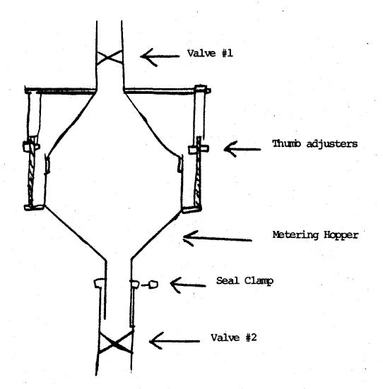
By thumb nut adjusters (3) the volume of the metering hopper could be changed thereby facilitating the selection of whichever concentration one desires.
