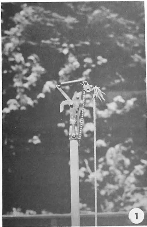
Figure 1. A clamping device attached to the head of a sectional pole pruner. Figure 2. A clamped branch sample; sample is released for free-fall to ground.
