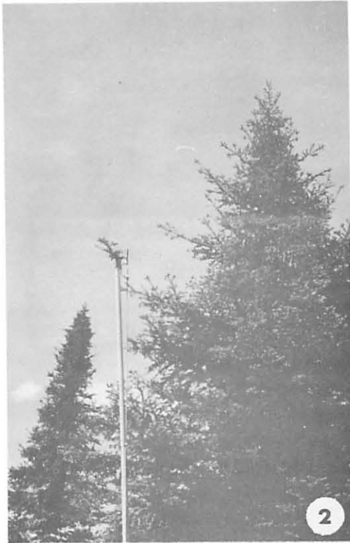
Figure 1. A clamping device attached to the head of a sectional pole pruner. Figure 2. A clamped branch sample; sample is released for free-fall to ground.
