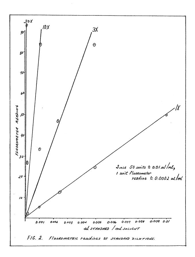
Since the 1X line in this case is the most accurate, use this fluorometer power in reading the experimental samples. Determine the unit fluorometer reading from the line. You will need this figure in deposit calculations.
