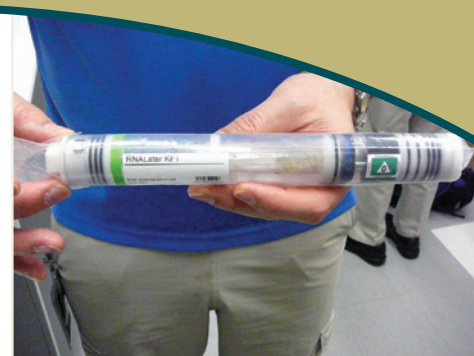
Tube developed at Kennedy Space Center for chemical fixation of biological samples in weightlessness conditions. Source: NRCan
