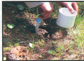
Installing Soil Collar
