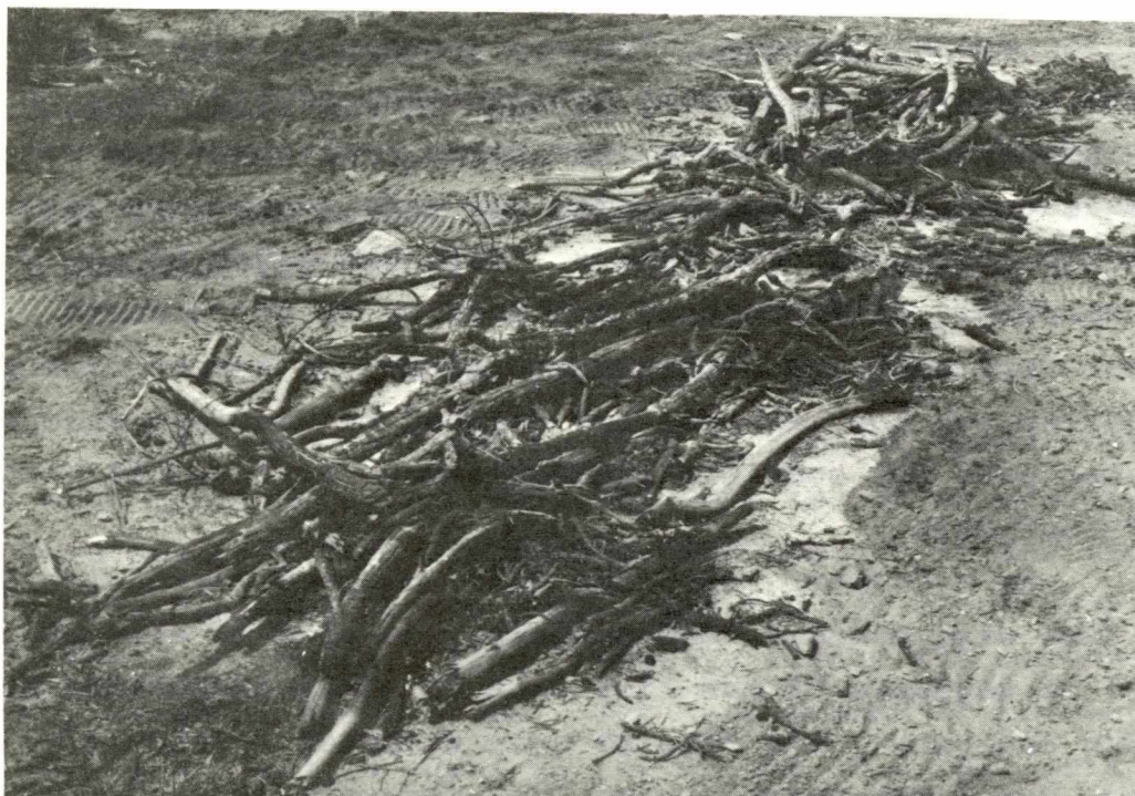
Figure 2. Crib after fire extinguished showing unburned fuel.
