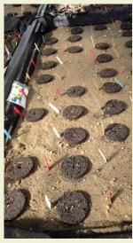
The pucks have been placed on two different soil types (clay loam and sand) to determine if soil medium has any impact on puck performance (above). By the end of the experiment, the team hopes to further narrow the puck recipe and better understand how the recipes impact germination and early establishment of plants.
