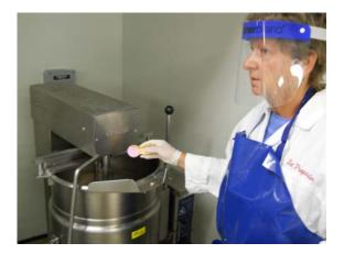
(b) The mixer motor shall be turned on and the heat turned on to setting 8-9 until the agar remnants begin to loosen.
