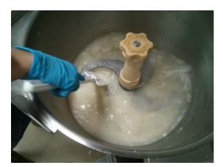
iv) Close the lid and run the motor on the "low" setting for about 1 minute to ensure complete mixing. While mixing, turn the handle manually to ensure that ingredients don't adhere to the mixing paddle.
