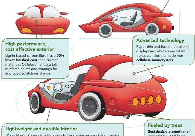
Wood fibre mats mould into products like dashboards and door panels that are 40% lighter than current materials. Cellulose nanocrystals or lignin-based bioplastics produce strong yet lightweight interior components like door handles and instrument panels.
