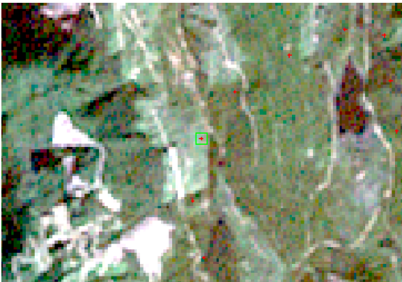
Landsat: It is often difficult to distinguish between tall and low shrub. A rule of thumb is that if the pixel is a green- brown colour as opposed to a more solid green colour then the pixel is low shrub.
