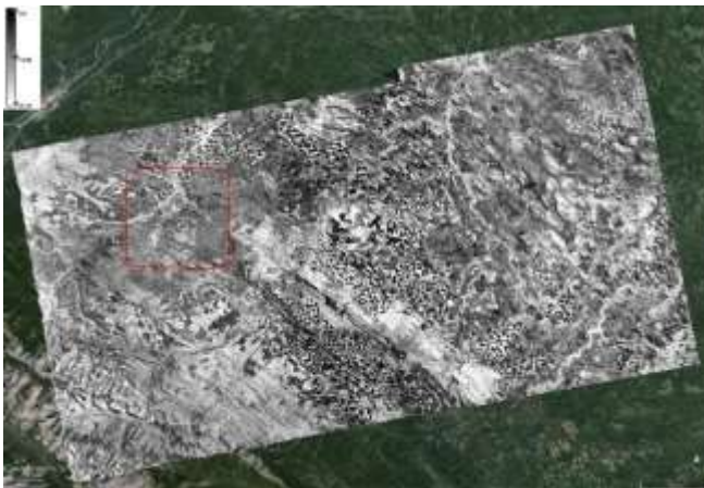
Figure 4: Wide area radar canopy height product over Hinton by using three TanDEM-X overlapping swaths (LIDAR in red)
