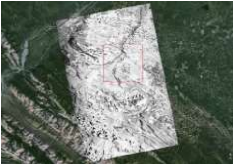
Figure 1: A coherence product (black=0, white=1) from 29/08/11 for Hinton with LIDAR coverage in red (15×15km 2 )
