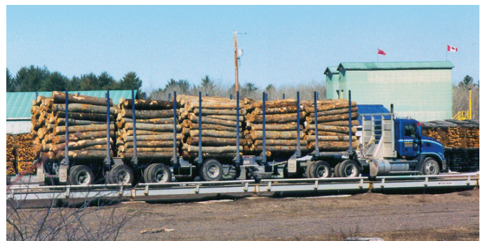
Truck loaded with logs on a weigh scale. The volume of logs is calculated from the weight of the load on the truck.
