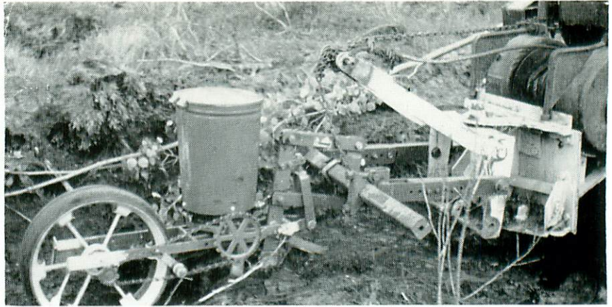
Close-up views of seeding unit showing it elevated for travel and, right, how it's bolted to tractor.
