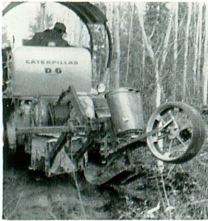
Close-up views of seeding unit showing it elevated for travel and, right, how it's bolted to tractor.
