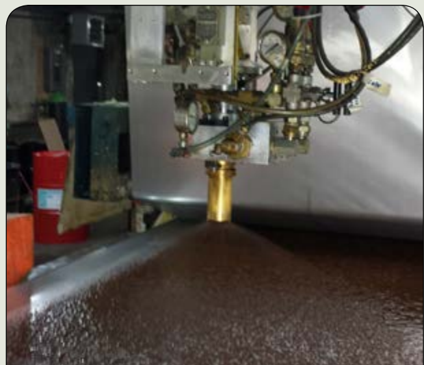
Iso-Lignin foam being sprayed to create a high-performance insulation board with customizable properties such as fire resistance and specific densities
