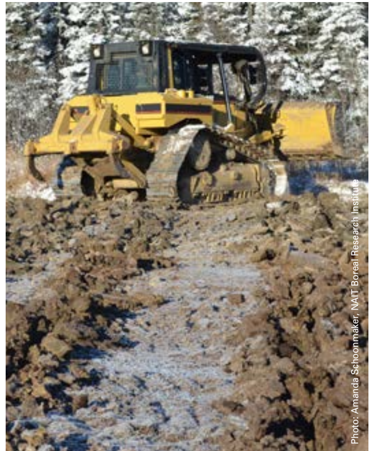
Figure 3. Straight ripper shank in the outside pockets of a multi-shank toolbar
