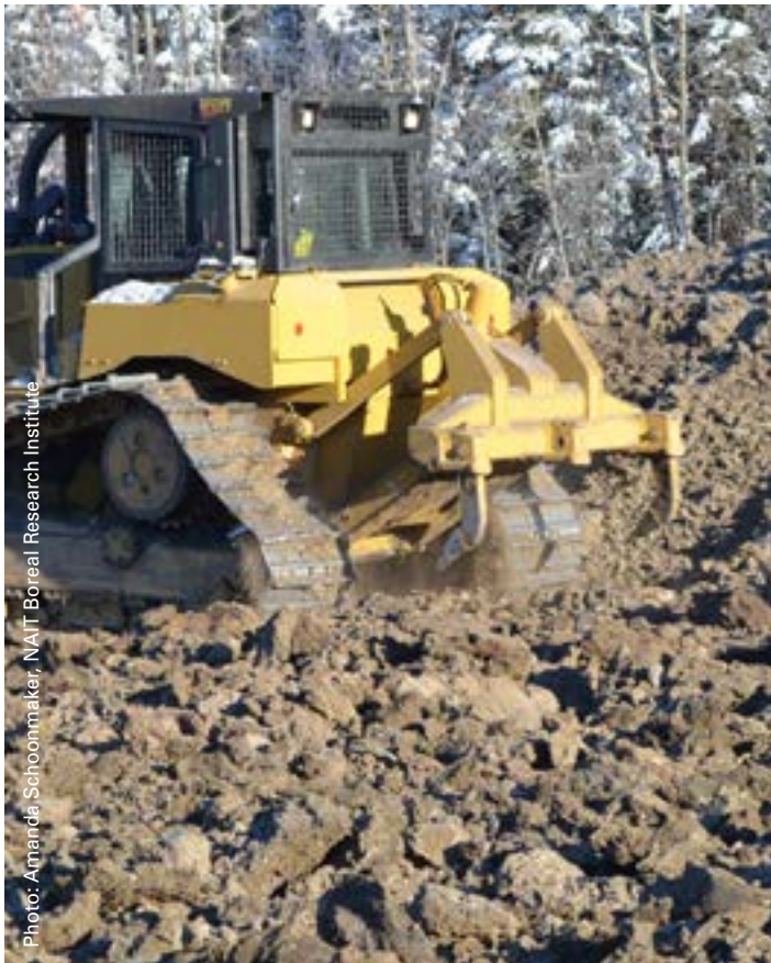
Figure 3. Straight ripper shank in the outside pockets of a multi-shank toolbar
