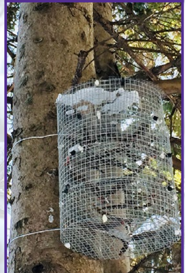
Galvanized wire crates, containing two branches. Four of these crates were assembled to form a tube, which, when installed on the tree, 2 m above ground, was used to test the winter survival of the SBW larvae.
