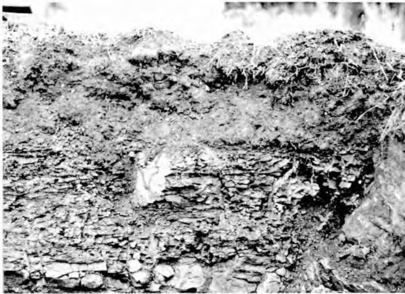
FIGURE 11 - Shale bedrock. Note the progressively smaller plates from bottom to top of the rock profile.
