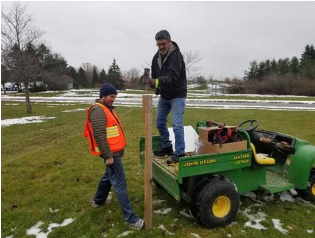
Installation of a CoCoRaHS rain gauge at GLFC.
