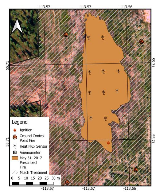
**Figure 2.** Overview of the experimental design, including heat flux sensor placement, ground control point fires, and the on-site anemometer location.
