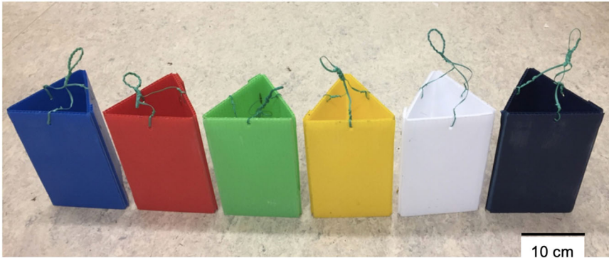
Fig. 2. Various colours of triangular prism trap used in the study. Left to right: light blue, red, green, yellow, white, and dark blue. Acadia University, Wolfville, Nova Scotia. Photograph by J. Goodwin.
