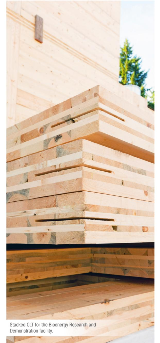
Stacked CLT for the Bioenergy Research and Demonstration facility.
