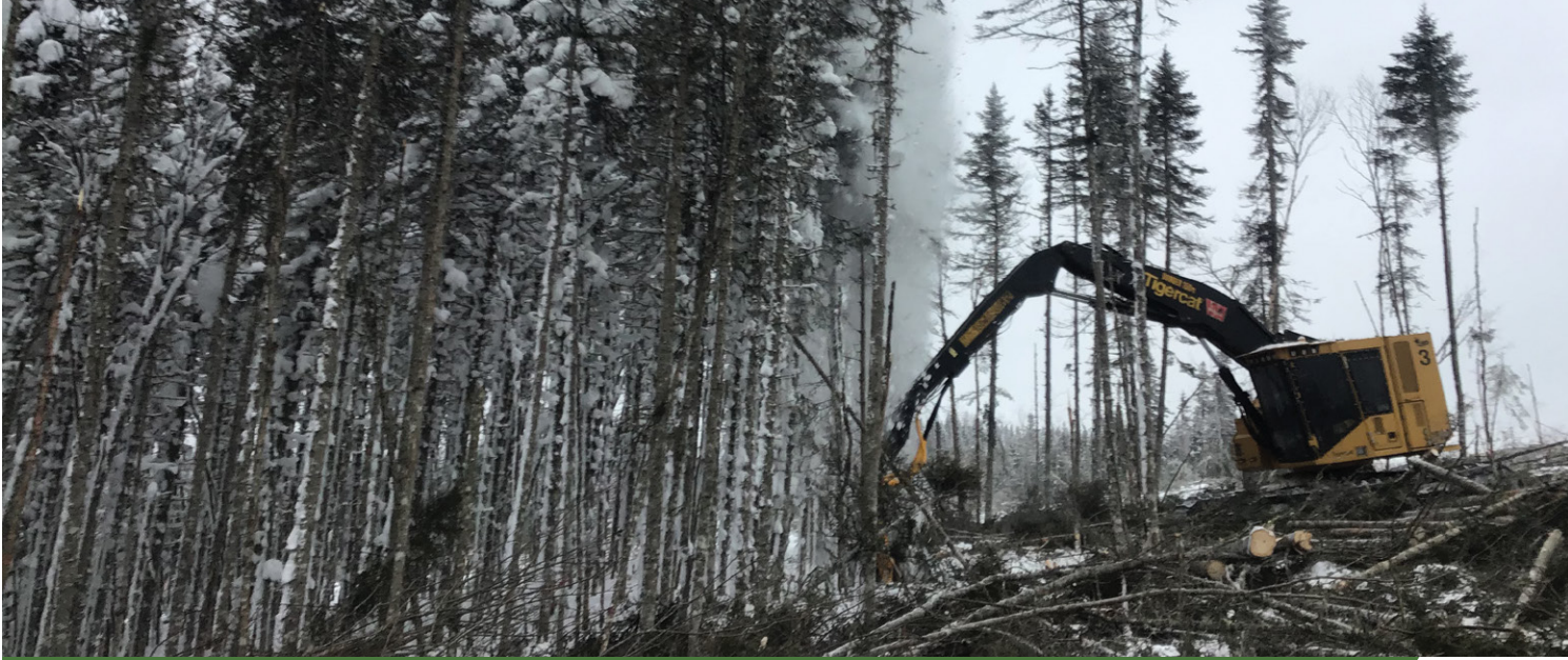
Figure 3. A harvester felling and processing trees into logs at the Nouvelle site (Photo by C.-M. Canuel).
