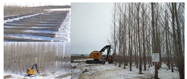
Figure 30. John Deere 753G Feller-Buncher at Eilerslie Short-Rotation Woody Crops Technical Development Site.
