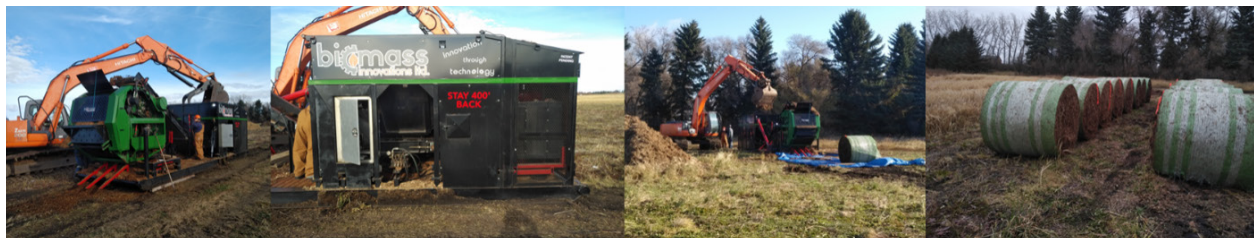
Figure 48. Woody biomass compaction unit prototype operational testing at Ellerslie Short-Rotation Woody Crops Technical Development Site.
