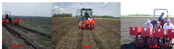
Figure 17. Mechanical transplanter configurations for 1, 2 and 3 row bed designs for the concentrated biomass plantation establishment.
