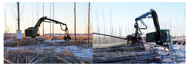
Figure 31. Timberjack 608 with Waratah processing head at Eilerslie Short-Rotation Woody Crops Technical Development Site.
