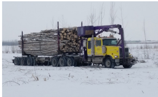
Figure 39. Self-loading log truck used at Ellerslie Short-Rotation Woody Crops Technical Development Site.
