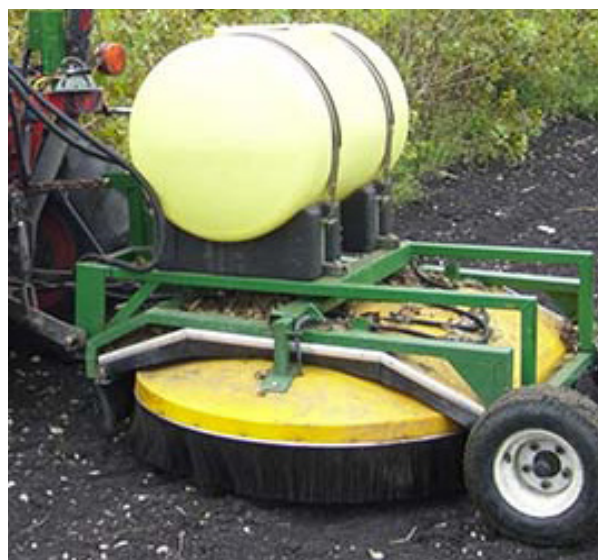
Figure 18. Enviromist shrouded herbicide sprayer.
